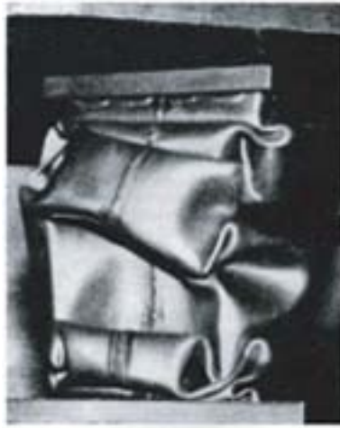
Fig. 2.4.1.2.1.2 Folding pattern of thin-walled box with very small thickness/width ratio
