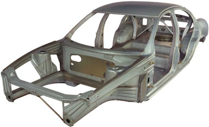
Fig. 1.2.2 Body-In-White image of a typical unibody construction
