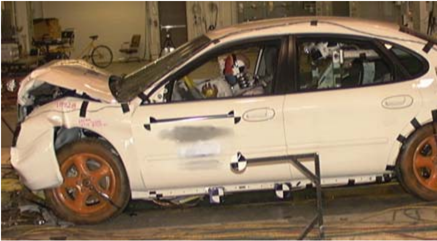
Fig. 4.2.1 Mid sized vehicle crash against a full rigid barrier
