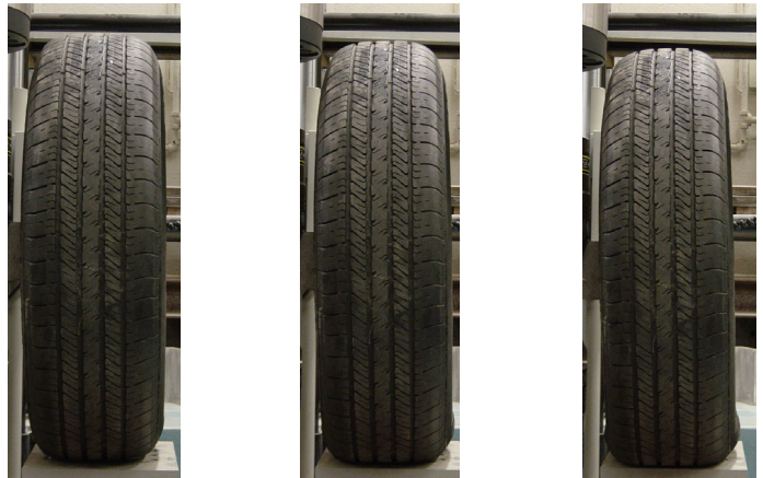
Figure 17: Comparison between the test and the simulation of the deformed shape at different loads.
