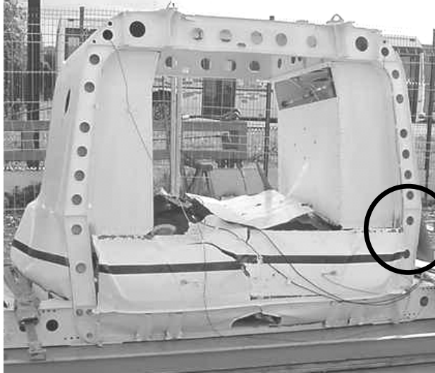
Main tank drop test results
