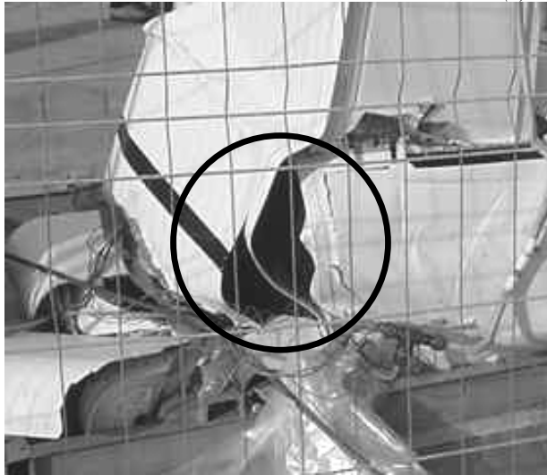
Main tank drop test results
