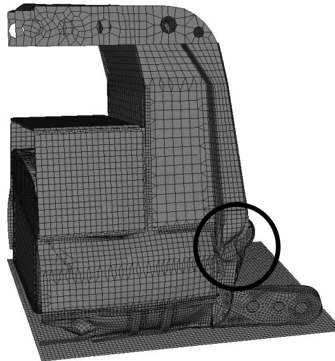
Main and auxiliary tanks simulation results
