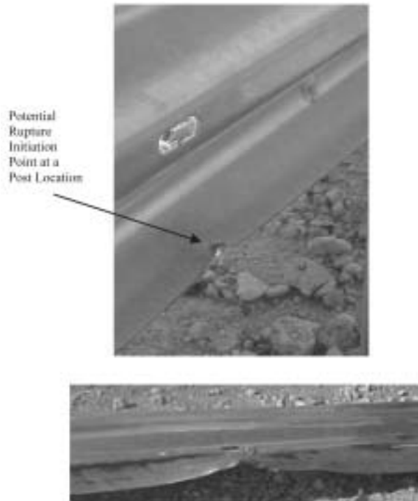
Figure 14. Picture of potential W-beam rupture initiation location.
