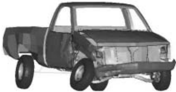
Figure 16. Damage to the vehicle after the second simulation study.
